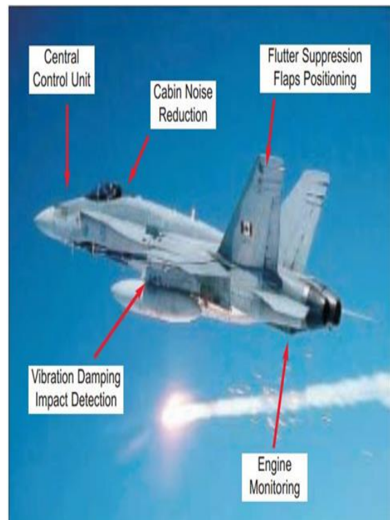
Fig.8: Positions of smarts materials in aircraft
